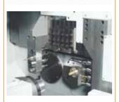
Various tooling(Max.18EA)Improved C/T and high productivity by horizontal type cross tool
